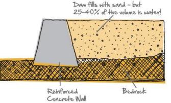
Sand accumulates behind the dam until it is full to the spillway. 25-40% of this volume is actually water, trapped in the spaces between grains of sand.
